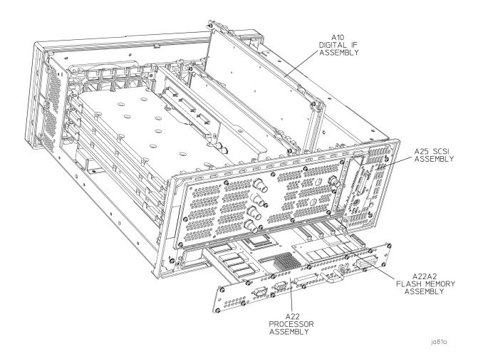
Figure 1. Replacing the Flash Memory Assembly
